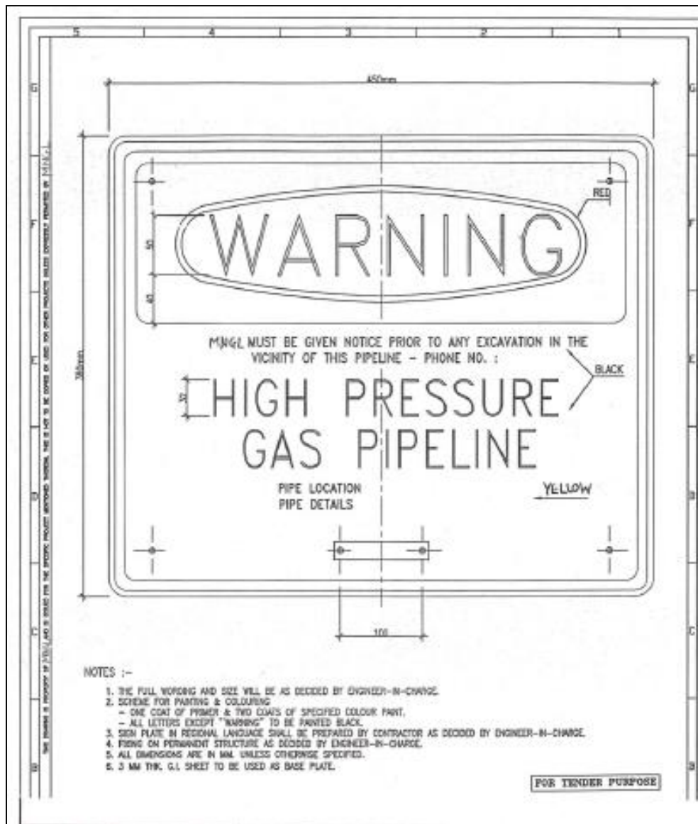
Warning Signs without foundation
