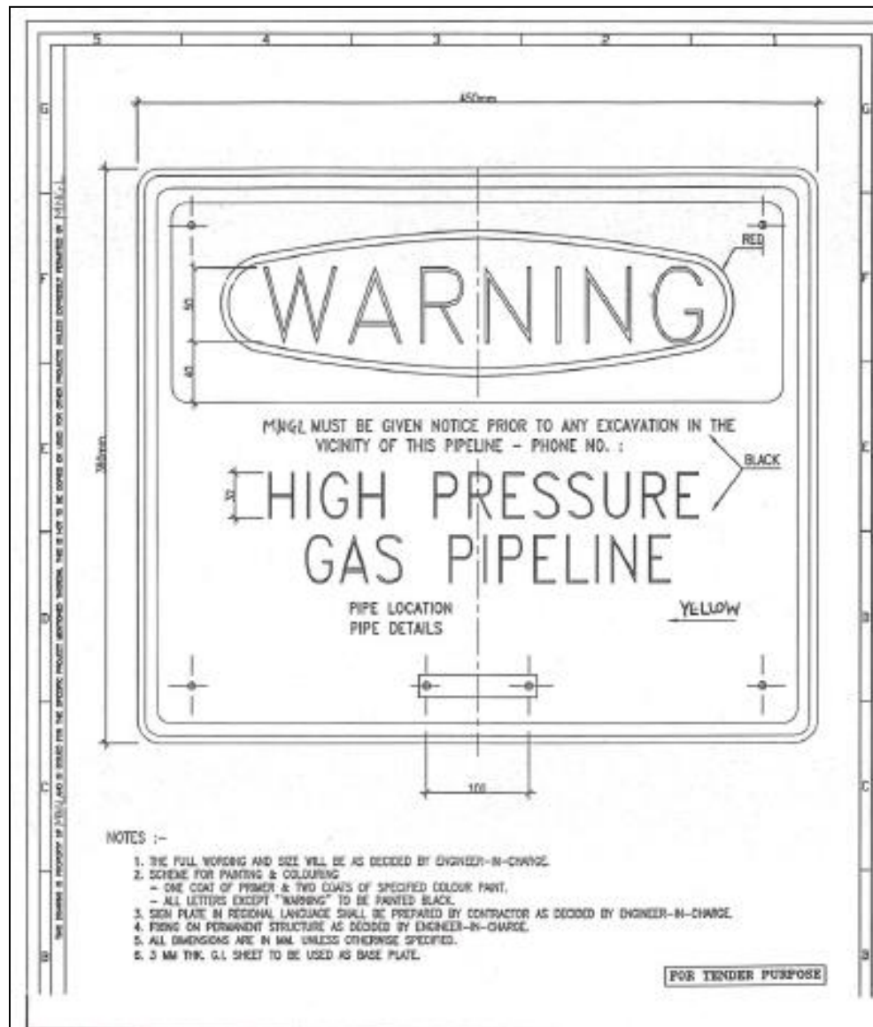
Warning Signs without foundation
